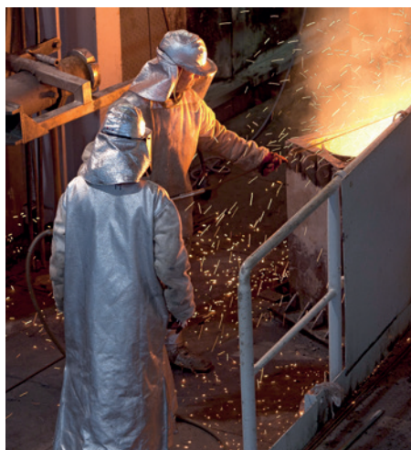
Pyrometallurgical processes convert used batteries into metal alloy (left); Steve Sloop has developed a method that produces fewer emissions and waste (right).
